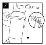
Turn off water and remove the service filter. Retain service filter for reuse. Fit new filter. Turn on water supply.
